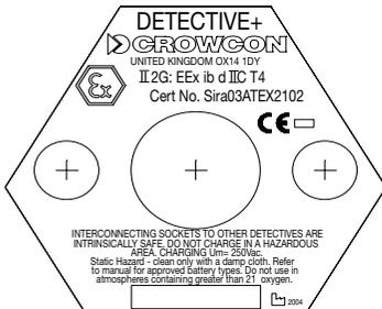
2. The equipment is Category 2G and may be used in zones 1 and 2 with flammable gases and vapours with apparatus groups IIA, IIB & IIC and with temperature classes T1, T2, T3 and T4
