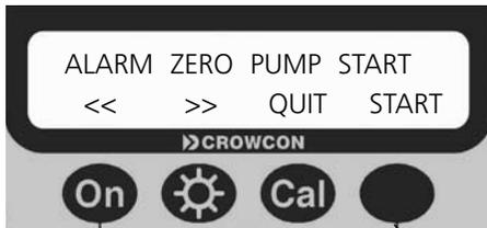
Press the UNMARKED button to enter the START submenu
