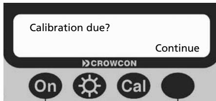
The instrument can alarm on instantaneous gas levels, and on both short and long term Time Weighted Average gas exposure levels. Note that the Time Weighted Average toxic gas exposures are reset to zero when the instrument is switched off.
