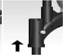
If the legs are too loose or are required to be permanently deployed, gently tighten the fixing bolt at the leg hinge.
