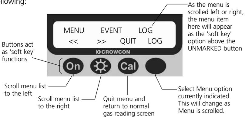
The four buttons have above them a symbol or word: these are the 'soft key' functions currently assigned to that particular key. Use the ON and BACKLIGHT buttons to scroll left and right, the CAL button to quit the menu system and the UNMARKED button to select a menu option. View the road map on page 37 for details of Detective+ configuration menu system
