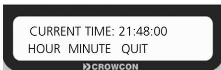
Press the key labelled HOUR to increment the hours and the key labelled MINUTE to increment the minutes until the correct current time is displayed
