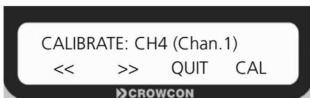
Use the first two keys to select the required gas. Press QUIT to move back up a menu level, or CAL to select the gas to calibrate. The display will now change to:
